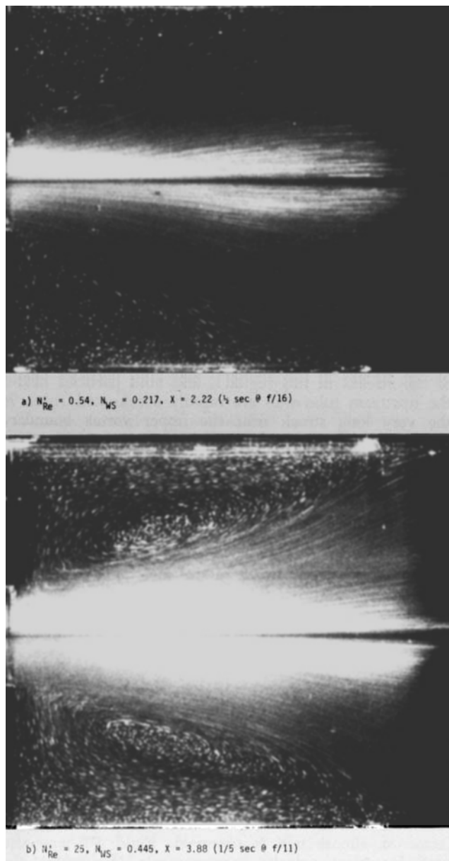
Fig. 7. Flow patterns upstream of the 4:1 contraction for fluid F9 at (a) 10.3 cm 3 /s and (b) 109 cm 3 /s.
